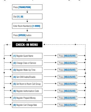
**Check-in** is performed directly from the **Attendant** keystation. Due to space availability on the LCD and the fact that you may not need to enter data against all the options each step in the menu is performed separately. Following the completion of each function the menu returns to the Check-in Menu where the next option is selected.
