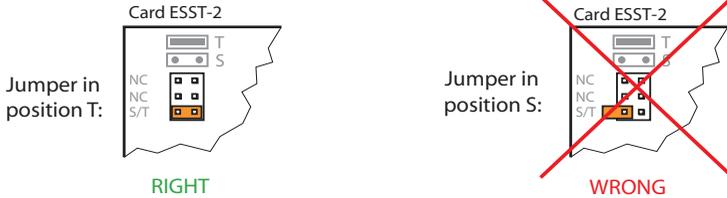
**Fig. 25** Jumper position on card ESST
