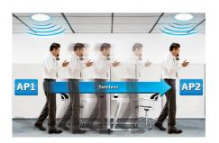
Samsung AirMove technology applies the handover methodology used within LTE mobile communications to deliver seamless roaming. Timing and choice of access point is determined centrally by the Access Point Controller (APC) which has a full picture of device activity and adjacent AP loading.
