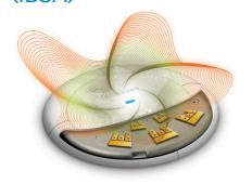
A Samsung 3 x 3 AP contains 14 antennas. Two antennas are used for RF monitoring and the remaining 12 provide an optimised RF pattern selecting a beam for each environment. As a result, dead areas are minimised, service coverage is expanded, and the receiving sensitivity is 2 dB higher than competitors' products. This means that the access point can accurately receive a signal from a mobile device with typically weak transmit power even when it is some distance away.
