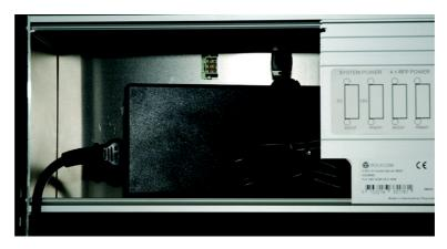
If more than two AC power adapters are used, these must be kept on a flat surface (same requirements as for the KWS8000 unit). In a rack installation the power adapters can be kept on a tray installed for the purpose provided that the ambient temperature is below 32°Celcius/89,6° Fahrenheit, and they have free air surrounding them.
