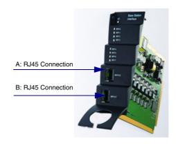
Figure 1-3 J45 Connections for AB Lines
