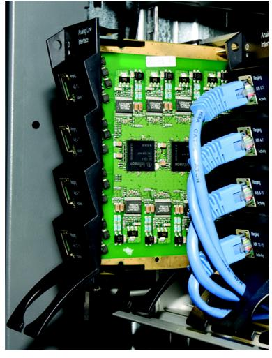
Figure 1-10 Installing Interface Cards
