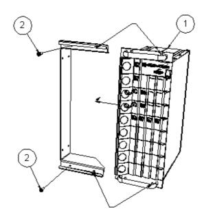
Installing the KWS8000 KWS8000 Installation
