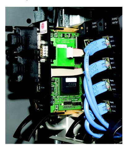
Figure 1-11 Installing CPU card
