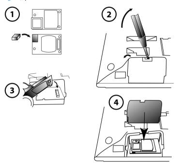
Fig. 68 Assembly of the Bluetooth module
