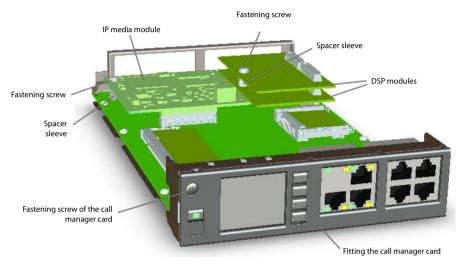
Fig. 27 System modules on the Call Manager card
