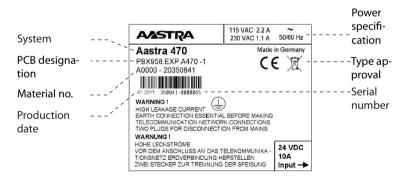
Fig. 87 Rating plate (example Aastra 470 communication server)
