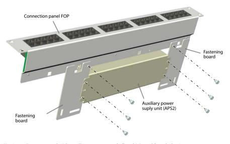
Fig. 25 Fan-out-panel with auxiliary power supply fitted (viewed from below)
