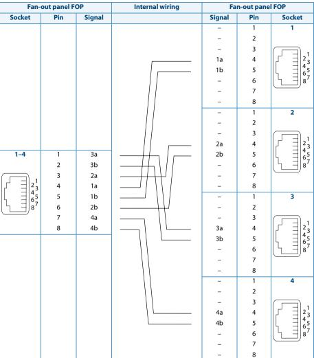
Tab. 70 Wiring of sockets 1-4 in the fan-out panel FOP
