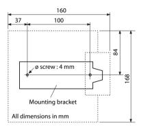
Fig. 71 Dimensional drawing for wall-mounting the mounting bracket
