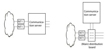
Fig. 29 Direct cabling (left) and indirect cabling (right)
