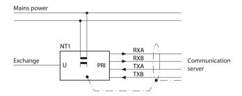
Fig. 40 PRI primary rate interface on NT1
