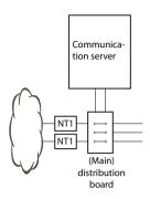
Fig. 30 Connection via main distribution board
