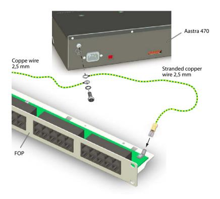
Fig. 65 Connection of the FOP fan-out-panel to the protective earth
