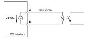
Fig. 60 Connection for FXS mode: Control output
