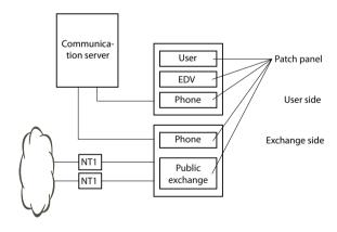
Fig. 33 Connecting to a UBC via wiring centre (example)
