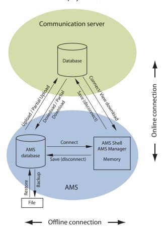
Fig. 75 Functions involved in exchange data between the communication server and AMS
