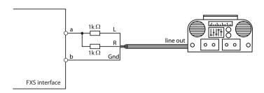
Fig. 59 Connection for FXS mode: External audio source
