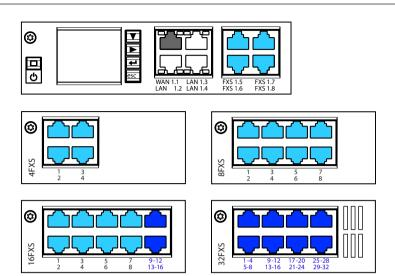
Fig. 56 Connection possibilities for FXS terminal interfaces
