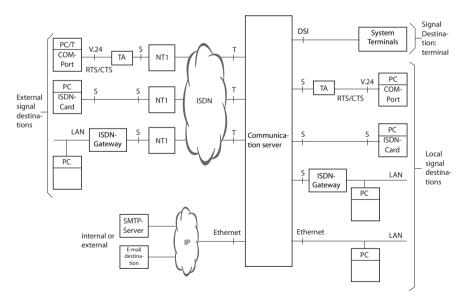
Fig. 84 Overview of connection possibilities for the various signal destinations
