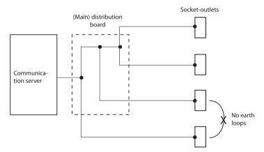
Fig. 23 Tree structure principle
