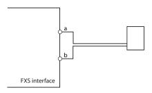
Fig. 58 Connection for FXS mode: Two-wire door
