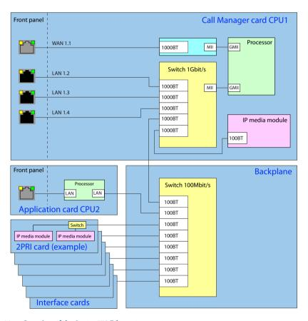
Fig. 11 Overview of the Aastra 470 Ethernet concept
