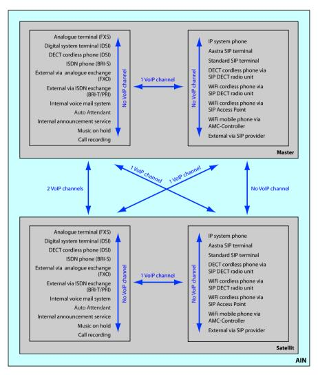
Fig. 13 Overview of the use of VoIP channels
