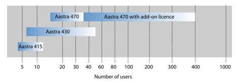
Fig. 2 Aastra 400 communication servers and their expansion capacity for IP system phones
