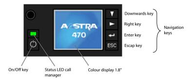
Fig. 80 Aastra 470 display and control panel
