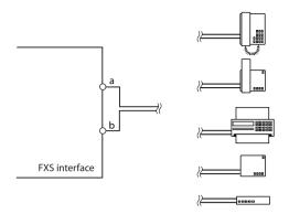
Fig. 57 Connection for FXS mode: Phone/fax
