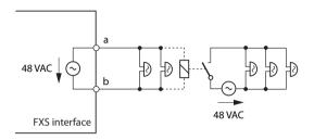
Fig. 62 Connection for FXS mode: General Bell
