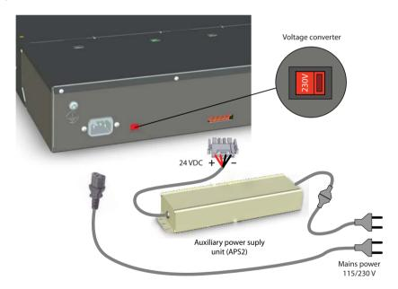
Fig. 24 Power supply to the communication server
