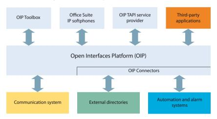
Fig. 3 OIP as middleware between communication system, external data sources and applications
