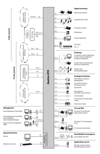
Fig. 4 Overview of interfaces with possible terminal equipment
