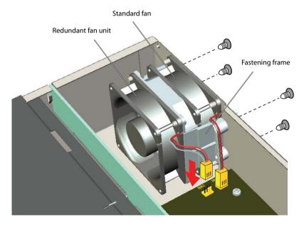
Fig. 20 Fitting the additional fan in Aastra 470
