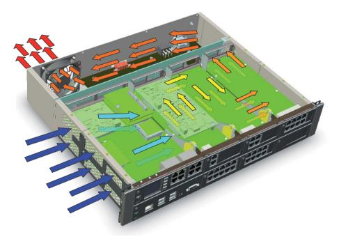
Fig. 19 Flow of hot air
