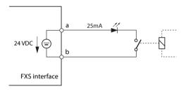
Fig. 61 Connection for FXS mode: Control input
