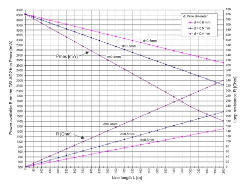
Fig. 48 Power available B on the DSI-AD2 bus
