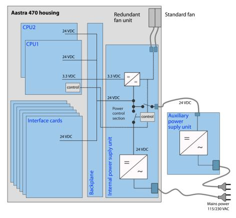
Fig. 10 Overview of the Aastra 470 power supply concept
