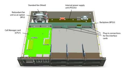
Fig. 7 Aastra 470 basic system fitted with a redundant fan unit
