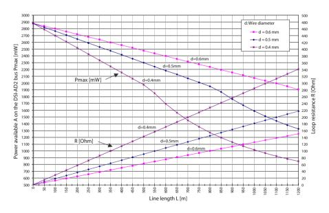
Fig. 47 Power available A on the DSI-AD2 bus
