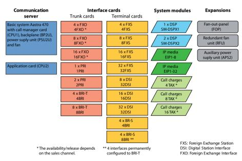
Fig. 5 Overview of the expansion possibilities
