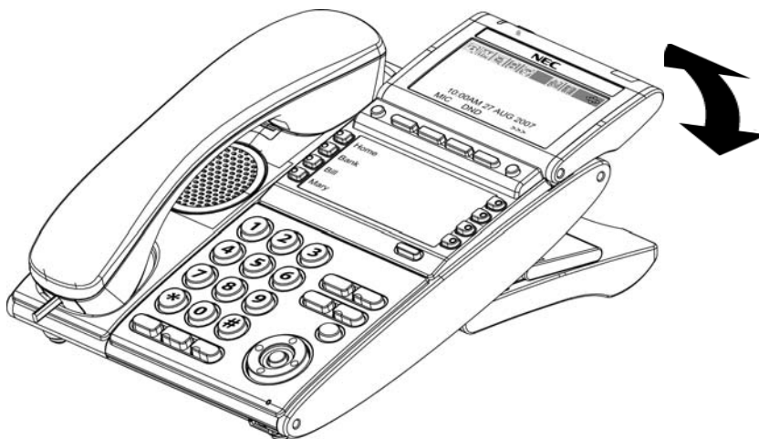
Figure 7-20 Adjusting the LCD on a multiline terminal
