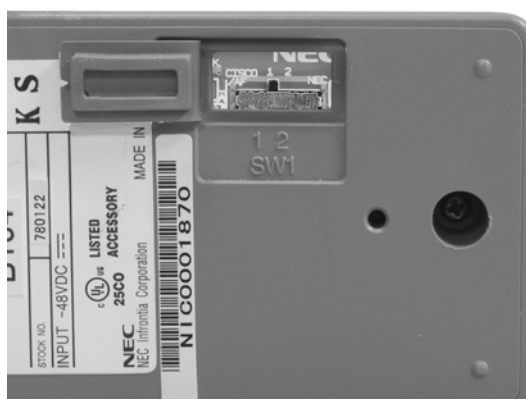
Figure 10-46 In-Line Power Adapter Switch Settings
