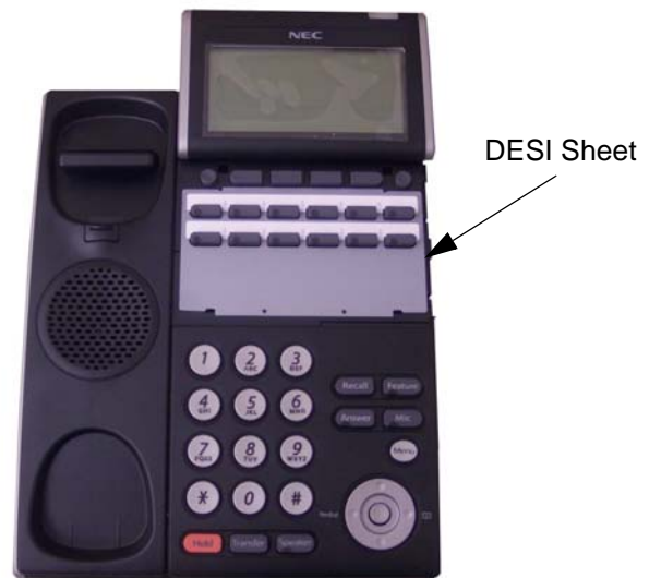
Figure 7-23 Removing the DESI Sheet
