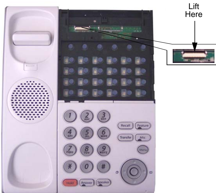
Figure 7-62 Ribbon Cable Connector
