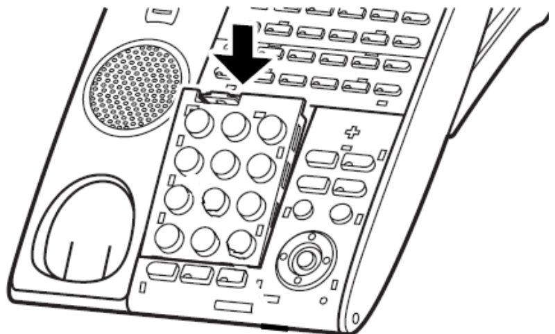
Figure 10-70 Install Numbered Keypad
