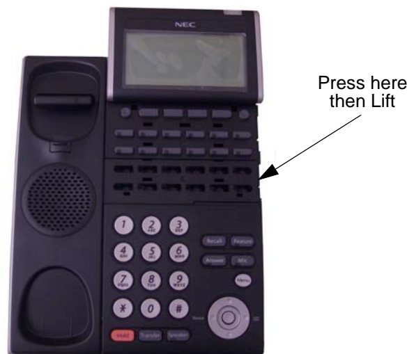
Figure 7-24 Removing the Line Key Placeholder
