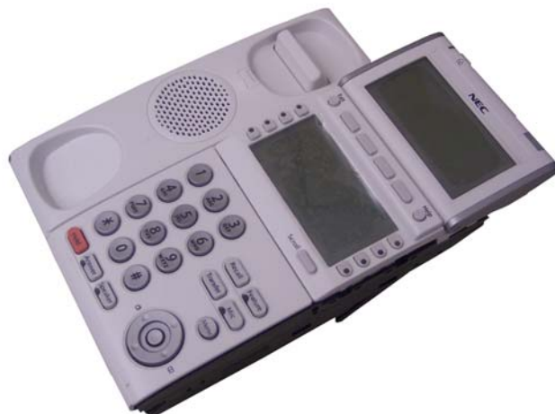
Figure 7-64 8LKI (LD)-L UNIT Installed
