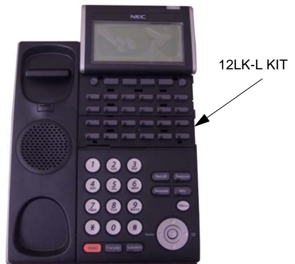
Figure 7-25 Installing the 12LK-L KIT
