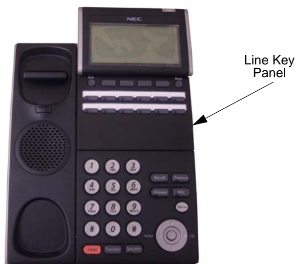
Figure 7-22 Removing the Line Key Panel
