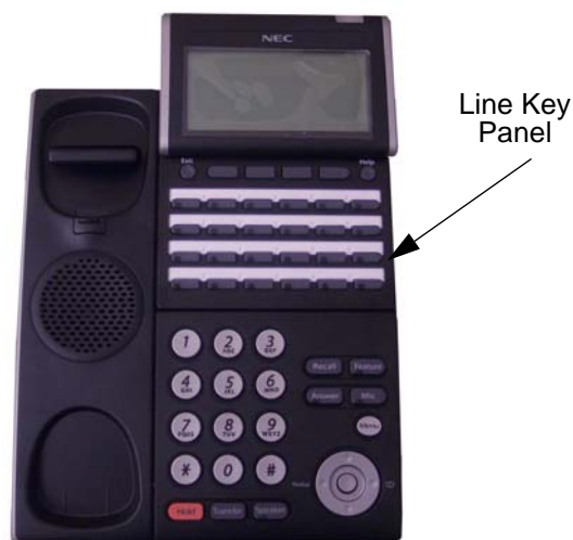
Figure 7-27 Installing the Line Key Panel
